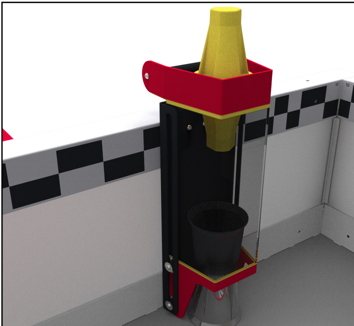
Figure SG11-1: Scoring Objects can be introduced through the top opening of the Loader.
