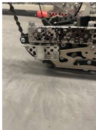
Figure 1: Wing mount on the side of the chassis
