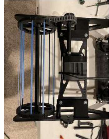
Figure 12: Front roller and chain mounted to the intake
