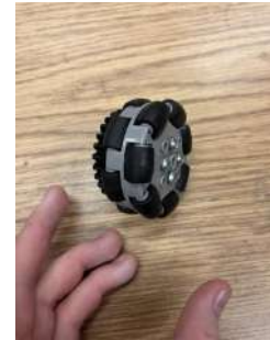
Figure 6: Vex IQ omni with gear hub assembly installed
