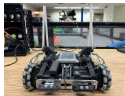
Figure 6: Chassis rear cross brace with wedge mounts
