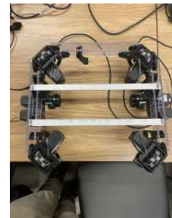
Figure 10: Cross braces attached to the chassis
