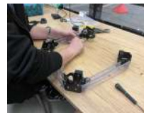
Figure 7: 3D printed wheel pods being attached to the polycarbonate frame pieces
