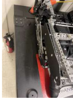
Step 9: Polycarbonate cover to protect the intake chain
