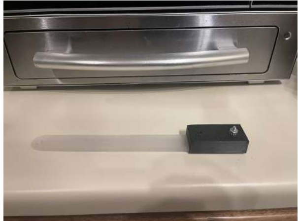
Figure 9: Intake bar with drilling jig
