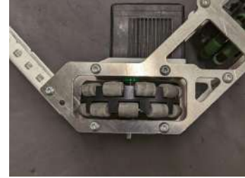
Figure 11: Wheels added to the chassis pods
