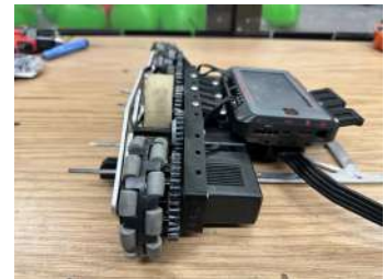
Figure 5: Inner chassis plate mounted with drive gears and motors
