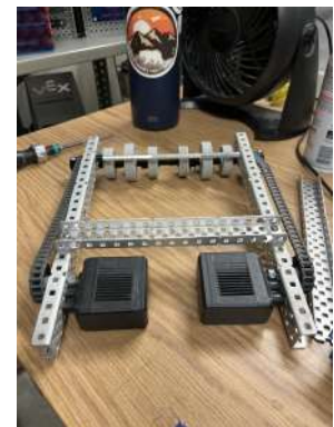
Step 5: Motors and chain on the intake
