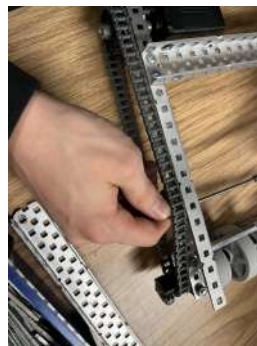
Step 5: Sprockets and chain run on one side of the intake
