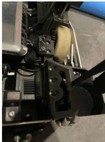
Figure 5: Tank and wing mount mounted to the inner chassis piece
