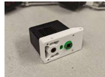
Figure 7: Motor attached to custom 3D printed mount
