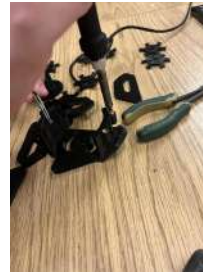
Figure 5: Soldering iron installed the heat sink inserts
