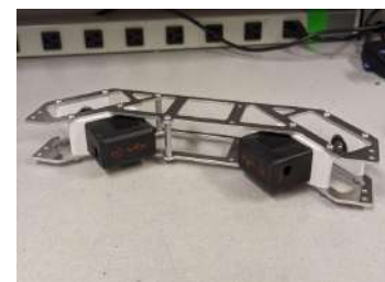
Figure 9: Motors mounted to the chassis frame
