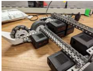
Step 6: Cross braces attached between the chassis halves
