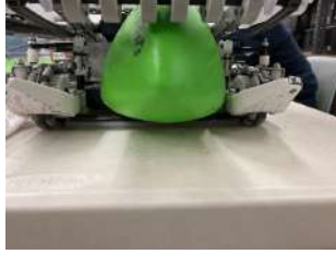
Triball in the completed intake
