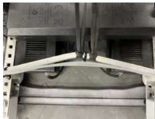
Step 5: added high strength axle cross brace and Triball support
