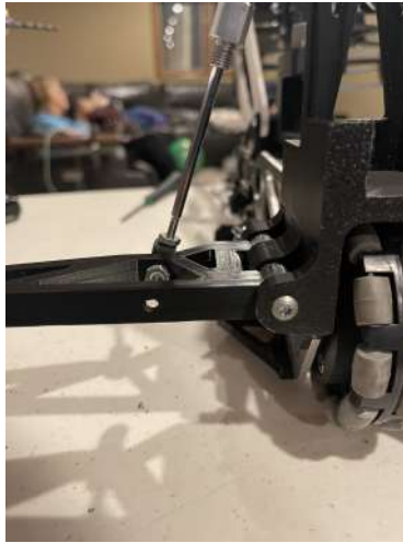
Figure 7: Extended Wing on the screw joint
