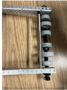
Steps 1, 2, and 3: Intake Axle attached to the intake bars
