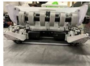
Step 6: Polycarbonate sleds added to the front of the intake
