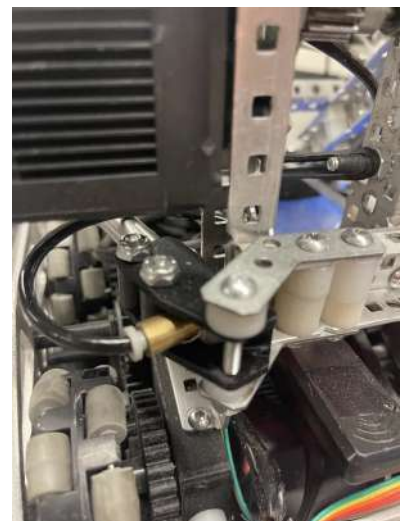
Figure 2: Piston mounted to the hang mechanism towers
