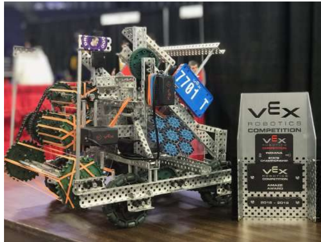
This is 7701T's Turning Point Robot. Turning Point was a VEX Game that required you to shoot balls at flags. The Rubber Band rollers shown grabbed the (significantly smaller) balls and primed them to shoot.
