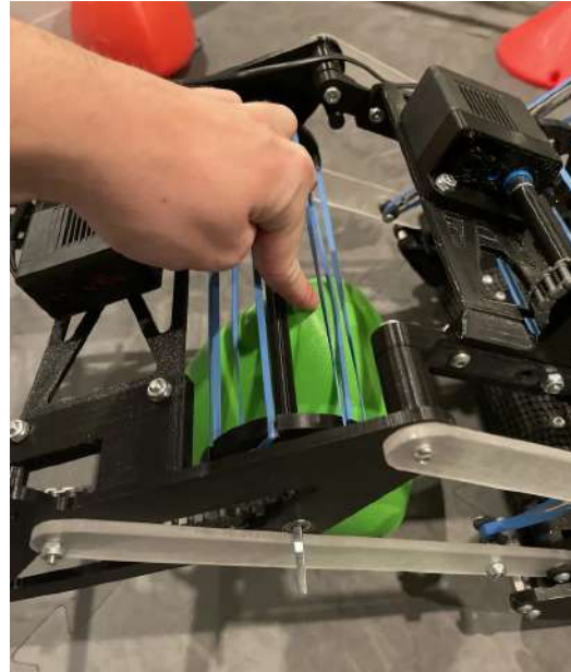
Figure 16: Triball as it moves through the intake
