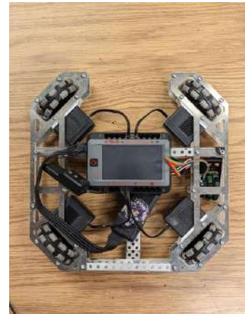
Figure 13: Completed chassis with brain attached for testing.
