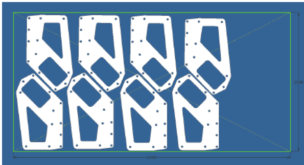
Figure 7: using a 12x24" sheet of aluminum, we can make all 4 pods.
