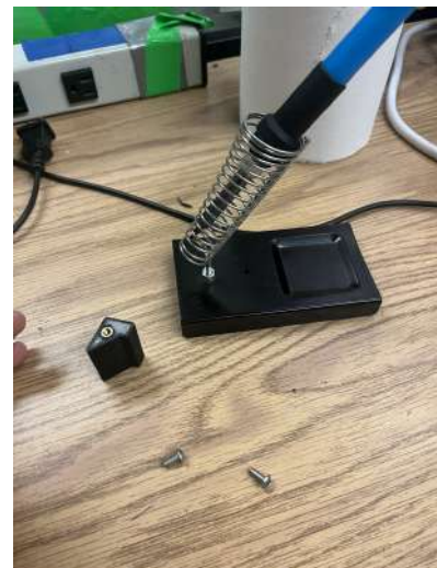
Figure 12: Inserting heat set insert with soldering iron
