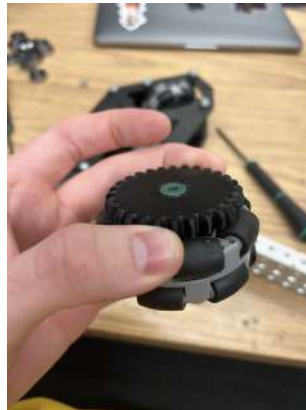
Figure 11: Wheel insert using thread in place screws
