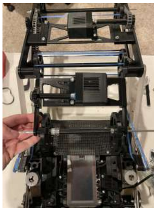
Figure 13: 3rd Roller Mount installed onto the intake cross bars
