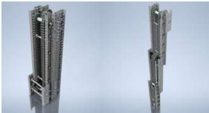
Figure 3: Cascade Lift Design from 99904A's Tower Takeover Robot
