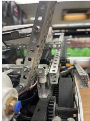
Step 1: Elevation bar attached to cross-brace
