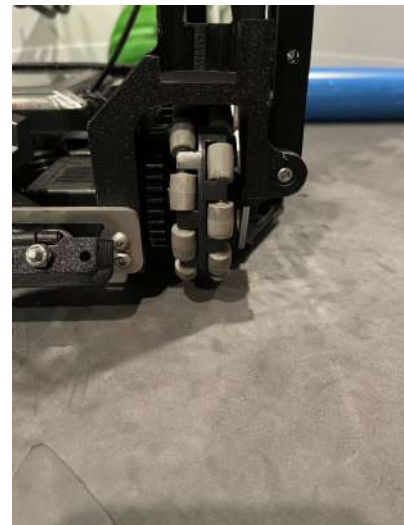
Figure 6: Rear mounting screws passing through the chassis brace plate
