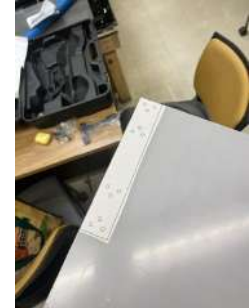
Figure 2: Template placed onto the polycarbonate sheet
