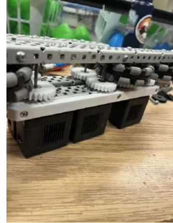
Steps 3, 4, and 5: Wheels and gears installed to inner and outer chassis supports
