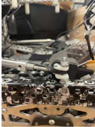
Figure 3: Piston mounted to the wing
