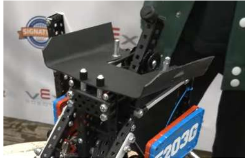
Figure 3: Kicker mechanism - 5203G
