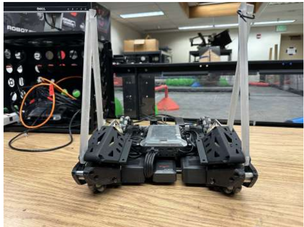
Figure 10: Intake mounts installed onto the chassis with intake arms
