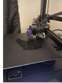
Figure 1: Conner's Ender 3 printing a motor mount to attach to the chassis
